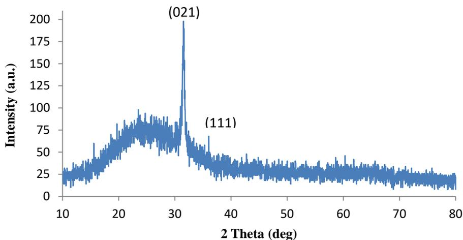
Fig. 1: XRD spectra of SnS thin films deposited on glass substrate.
