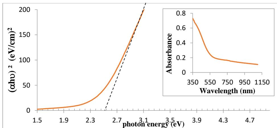
**Fig.5** Optical Absorbance of SnS thin films and  $(\alpha h\nu)^2$  versus photon energy gap plot
