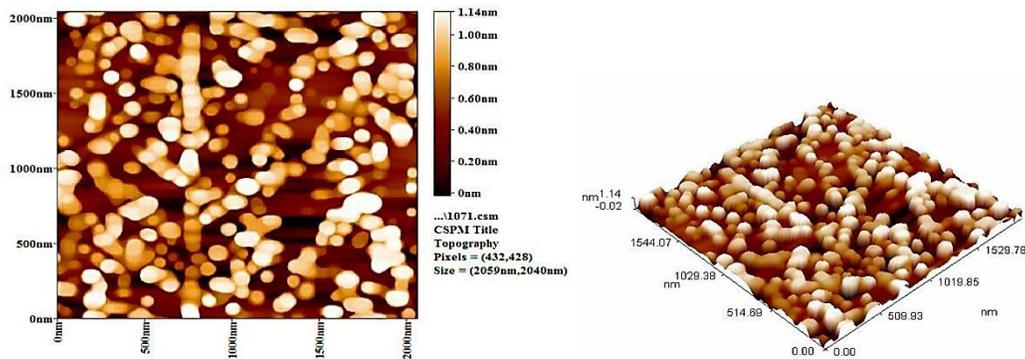
Fig. 3:AFM images and granularity accumulation distribution chart of SnS thin .
