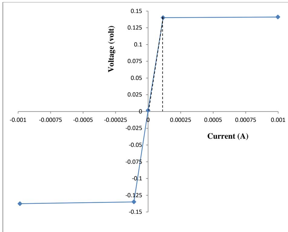
Fig. 7 Room temperature  $I$ - $V$  characteristics of Al/SnS/Al nanoparticles contact
