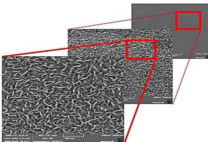
Fig. 2 SEM images of SnS nanoparticles prepared with laser energy 400m J .(magnified images )
