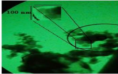
*Fig.4 TEM of SnS colloidal nanoparticles dissolved in water and prepared with 400 mJ laser fluence.*
