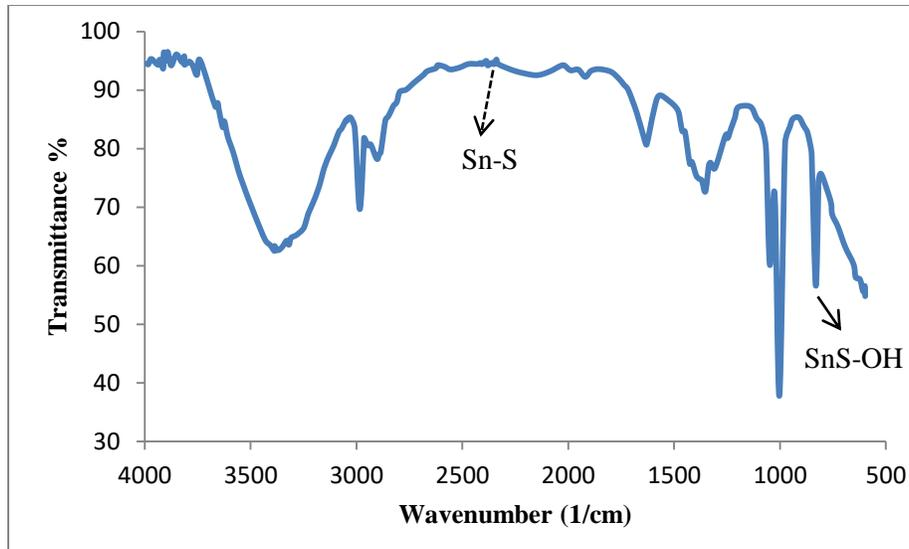
Fig.6: FTIR spectra of SnS thin film
